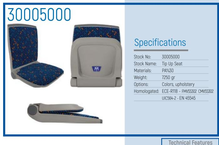
All the plastic materials in this parts are in conformity with the specifications and REACH. All the physical loading tests are done. In design we focused on creating robust, ergonomic, innovative, compact plastic seat. The seat is designed customizable. The tip-tip seat has passed 1.000.000 cycle test and 350 kg static loading test successfully.
